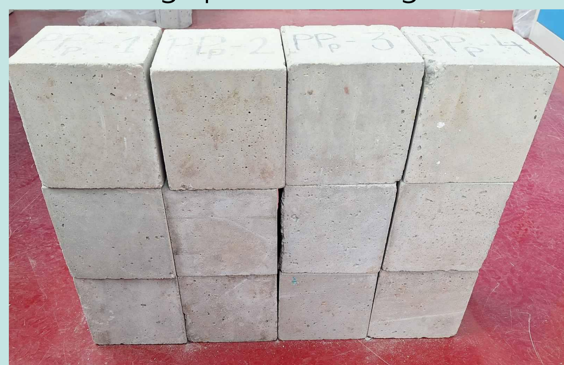
Figure 2. Prepared concrete specimens from the same batch for quasi-static compression testing
