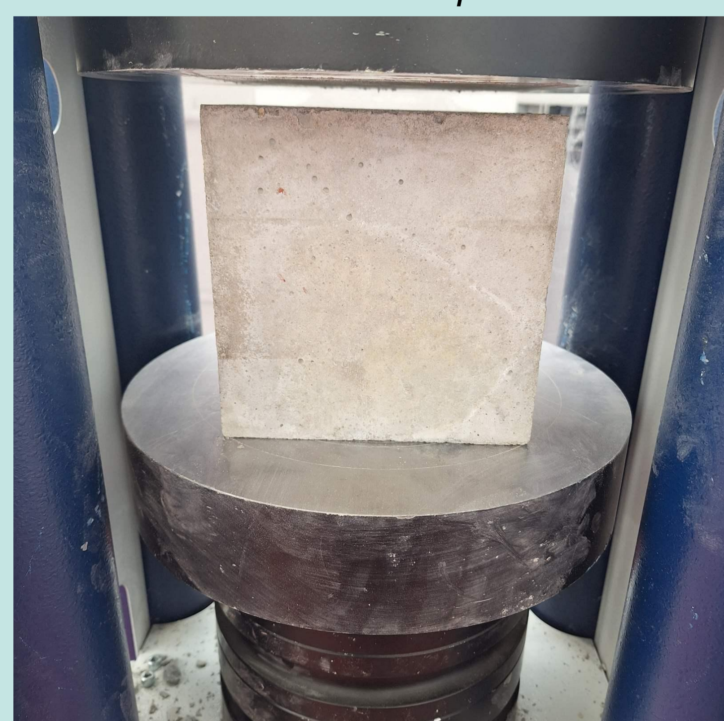
Figure 3. Concrete specimen positioned in the hydraulic press prior to testing – left; Concrete specimen after compression testing, showing crack formation and failure – right
